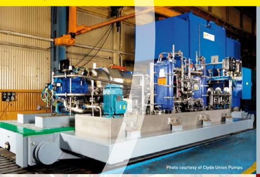
ATB LS Frame PA630 2950kW, 3950HP 2 pole 13.8kV 3ph 60Hz IP56 Ex e px II T3 Clyde Union Pumps offshore Angola
