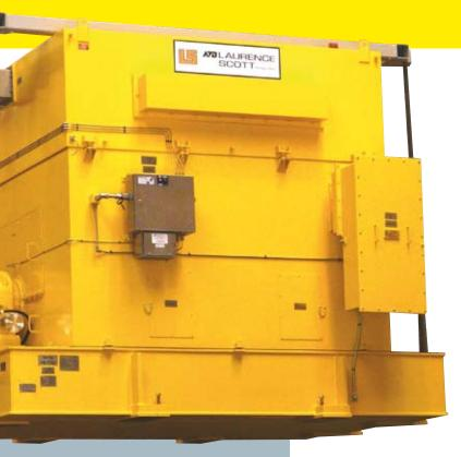
11566kW, 15500HP 4pole 11kV 3ph 60Hz TEWAC/CACW IP56 Ex e px II T3 Designed for 300% Starting Current
