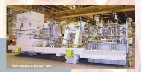
An ATB LS compressor drive for the Petrobras FPSO, Cidade de Angra dos Reis MV22. ATB LS Frame PL 710 5450kW 7300HP, 4pole TEWAC/CACW IP56 11.0kV 60Hz In standard form, ATB LS machines are manufactured in accordance with IEC 60034-1. Where specified, however, machines can be supplied to meet NEMA, API and other national and international standards, as well as contractors' and end users' specifications.
